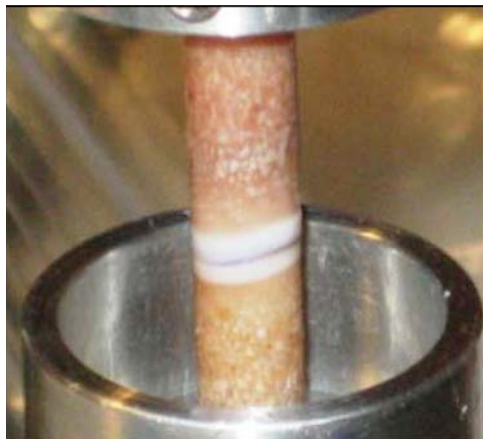
Fig. 2 Setup showing the mated cartilage on cartilage osteochondral plug harvested from patella-femoral joint.
